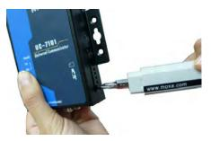
**Step 2:** After removing the cover, insert the SD memory card into the slot.
