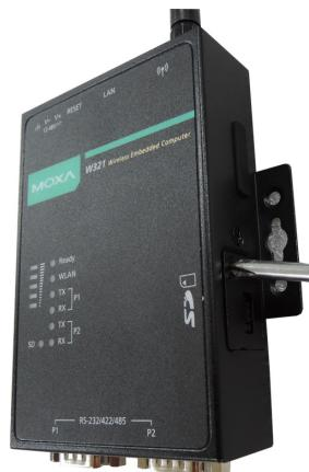
**Step 2:** After removing the cover, insert the SD memory card as shown.
