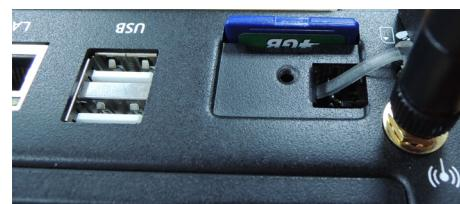
**NOTE** To remove the SD memory card from the slot, press the SD memory card in slightly with your finger, and then remove your finger to cause the card to spring out partially. You may now grasp the top of the card with two fingers and pull it out.
