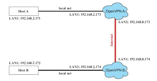
The configuration procedure is almost the same as for the previous example. The only difference is that you will need to indicate the #up parameter. "/etc/openvpn/A-tap0-br.conf" and "/etc/openvpn/B-tap0-br.conf".
