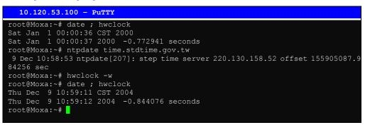
**NOTE** Before using the NTP client utility, check your IP and DNS settings to make sure that an Internet connection is available. Refer to Chapter 2 for instructions on how to configure the Ethernet interface, and see Chapter 4 for DNS setting information.
