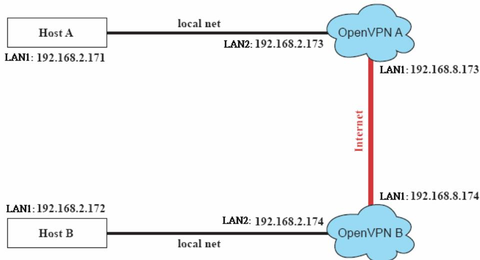
2. The configuration procedure is almost the same as for the previous example. The only difference is that you will need to comment out the parameter `up` in `/etc/openvpn/tap0-br.conf` of OpenVPN A and `/etc/openvpn/tap0-br.conf` of OpenVPN B.
