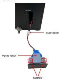
4. Separate the connector and remove the two screws on the metal plate.
