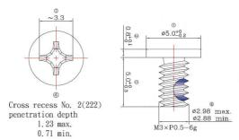
Use 2 screws (M3\*5L standard is recommended) on each side to attach the V3200 to a wall or cabinet. These 4 screws are not included in the product package; they need to be purchased separately.
