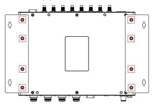
The 8 screws for the mounting brackets are included in the product package. They are standard IMS\_M3x5L screws and require a torque of 4.5 kgf-cm. Refer to the following illustration for details.
