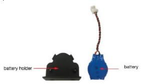
Replace the new battery in the battery holder, place the metal plate on the battery, and fasten the two screws tightly.
