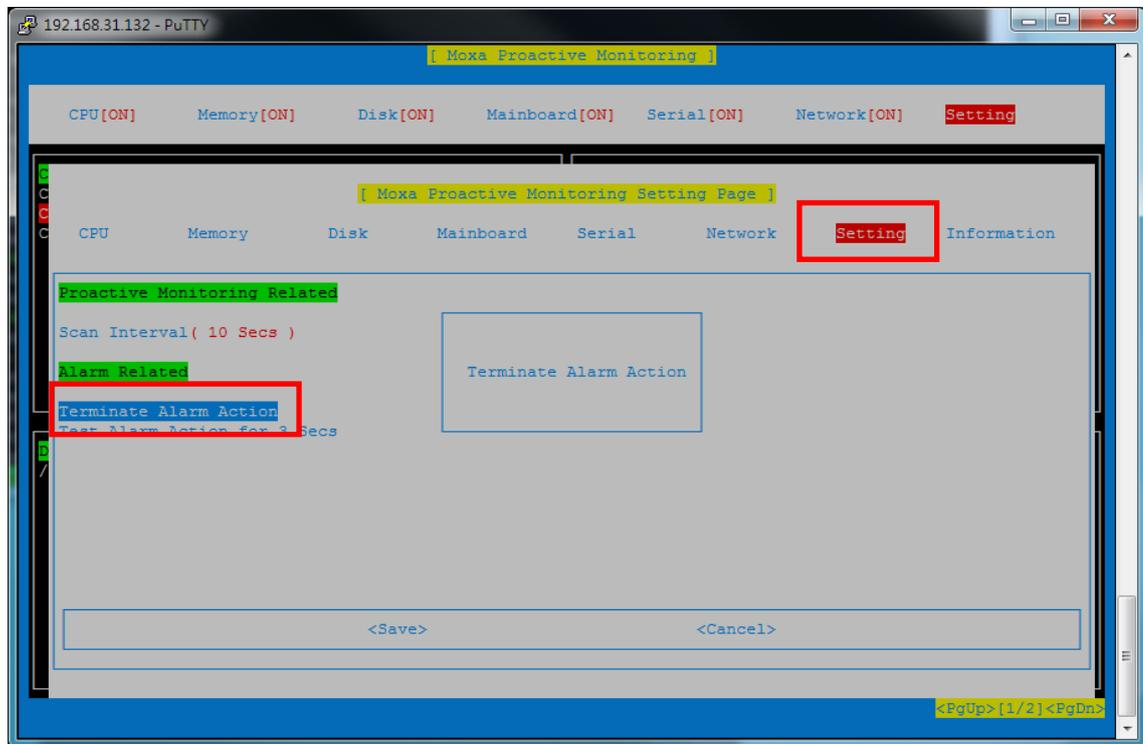
2. Terminating an alarm action will execute the `/sbin/mx_stop_alarm` file. You can edit `/sbin/mx_stop_alarm` to change the stop alarm action. The script will set the first digital output to low in the default setting.
