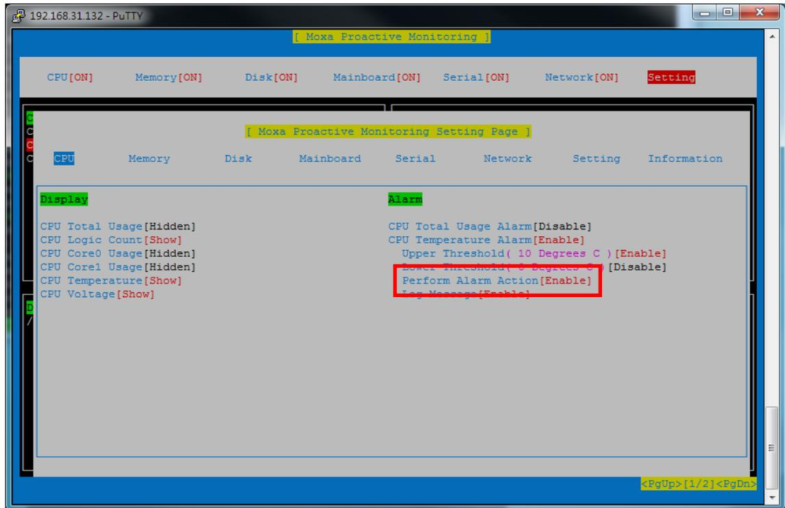
2. After you save the setting, Moxa Proactive Monitoring will perform the alarm action when the alarm occurs. You can edit **/sbin/mx\_perform\_alarm** to change the alarm action. The script will set the first digital output to high in the default setting.
