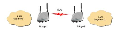
It is a good idea to plan your wireless network by drawing a diagram so that you know how each AWK-4121 is connected to other peer APs or wireless bridges by WDS, and how bridges are connected to other peer bridges by WDS. See the following figure for an example of a network-planning diagram.
