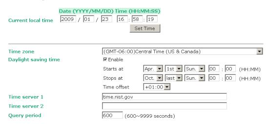
**Current local time** shows the AWK-4121's system time when you open this web page. You can click on the **Set Time** button to activate the update after setting up the date and time parameters. An "(Updated)" string will appear to indicate that the change is complete. Local time settings will be immediately activated in the system without running Save and Restart.
