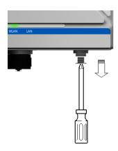
**STEP 2:**Using a pointed object, press and hold the reset
