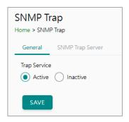
Set up the SNMP trap server to send the trap events, such as warning messages.
