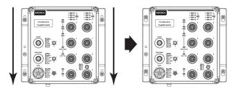
**NOTE** To provide greater protection from vibrations and shocks, use screws with shaft diameter between 6.0 mm and 7.0 mm, and fix the ToughNet switch onto the wall directly through the large opening of the keyhole-shaped apertures.
