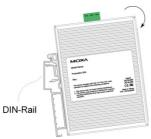
To remove Moxa EDS-205 from the DIN rail, insert a flat-blade screw driver horizontally into the DIN-rail kit under the EDS-205, and then pull it upwards and release the EDS towards you and away from the DIN rail.
