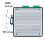
To remove the EDS-P510 from the DIN-Rail, simply reverse Steps 1 and 2 above.
