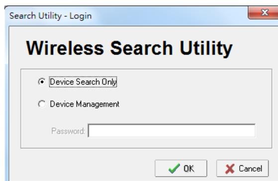
**NOTE** To apply device search and management, ensure your device at factory default setting or remove your SIM card. This is to avoid assigned IP different from default subnet and result in function failure.
