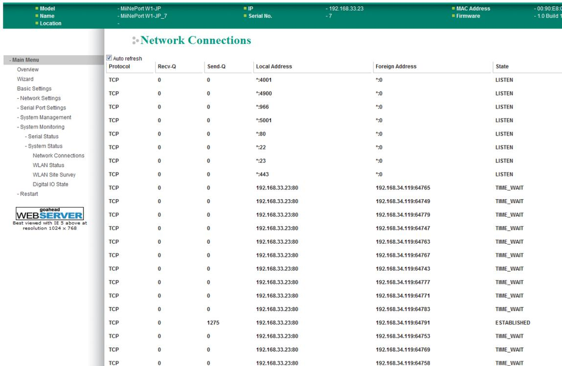
The **Network Connections** page is located under **System Status** in the **System Monitoring** folder. On this page, you can view the current status of any network connection to the MiiNePort W1/MiiNePort W1-T.
