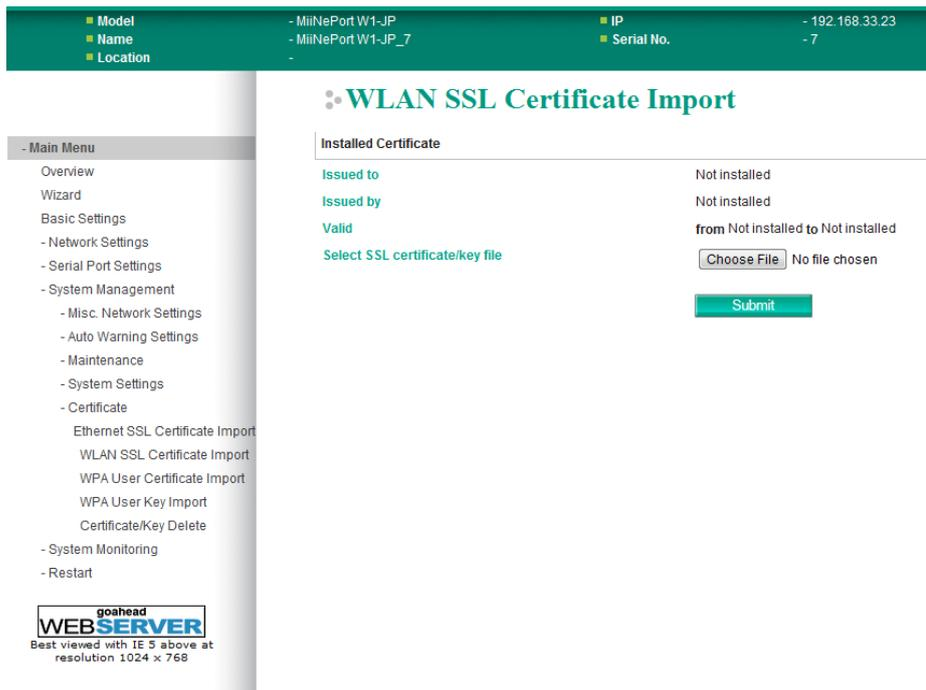
The **WLAN SSL Certificate Import** page is located under **Certificate** in the **System Management** folder. By default, the WLAN SSL certificate is automatically generated by the MiiNePort W1/MiiNePort W1-T based on the IP address of the wireless interface. You can also import a certificate. Select or browse for the certificate file in the **Select SSL certificate/key file** field.
