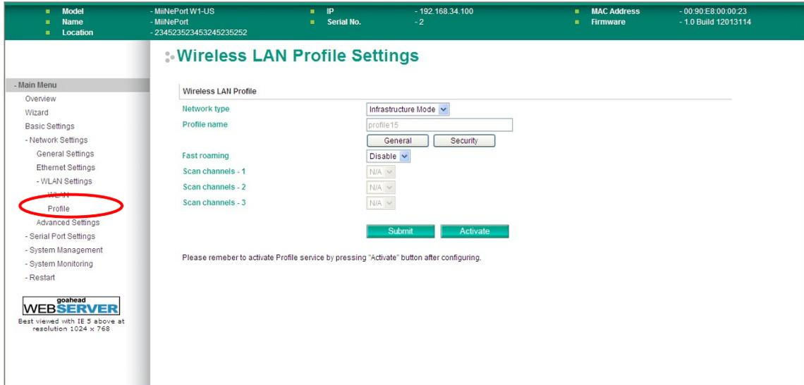
The **Profile** page is located under **WLAN Settings** in the **Network Settings** folder. This is where you configure the MiiNePort W1 series for Ad-hoc or Infrastructure operation. Different settings are available depending on whether you select Ad-hoc Mode or Infrastructure Mode.
