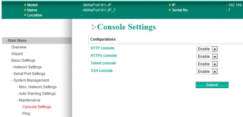
The **Console Settings** page is located under **Maintenance** in the **System Management** folder. This is where you enable or disable access to the various module configuration consoles. You may modify **HTTP console**, **HTTPS console**, **Telnet console**, and **SSH console**.
