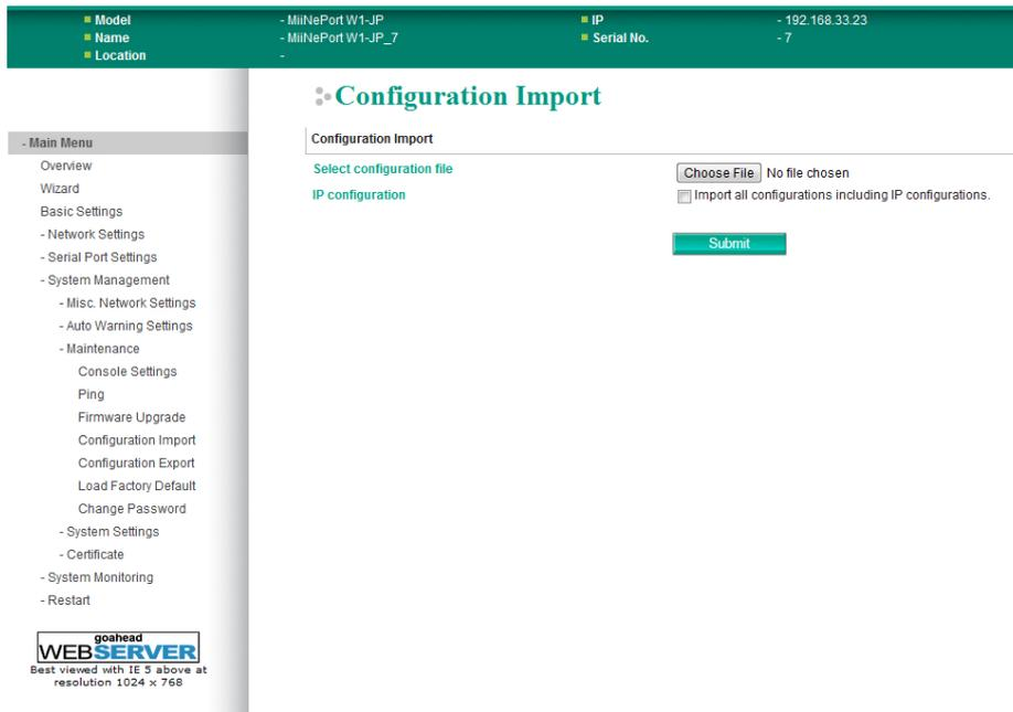
The **Configuration Import** page is located under **Maintenance** in the **System Management** folder. This is where you can load a previously saved or exported configuration. Select or browse for the configuration file in the **Select configuration file** field. If you also wish to import the IP configuration (i.e., IP address, netmask, and gateway), make sure that **Import all configurations including IP configurations** is checked.
