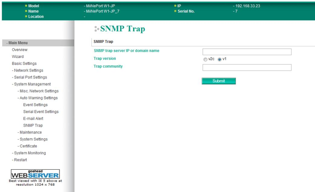
The **SNMP Trap** page is located under **Auto Warning Settings** in the **System Management** folder. This is where you specify the SNMP trap settings to use for automatic notification of system and serial port events.
