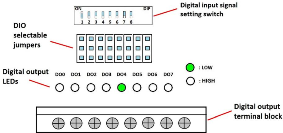
1. First, position the jumpers so they correspond with the input/output mode of each digital I/O channel. In the example below, channels 0 through 3 are output (DO) channels and channels 4 through 8 are input (DI) channels.
