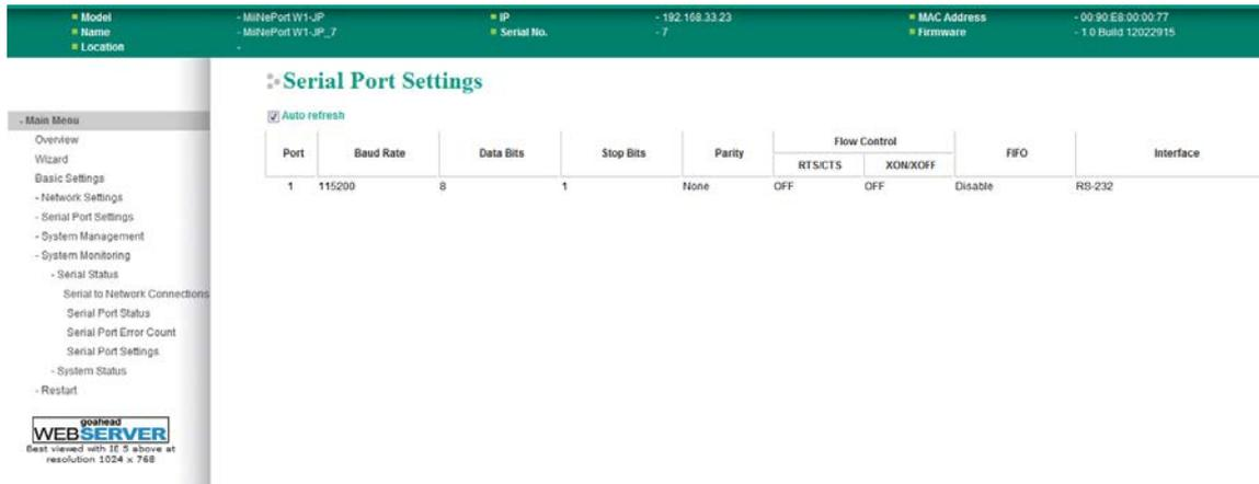
The **Serial Port Settings** page is located under **Serial Status** in the **System Monitoring** folder. On this page, you can view the current serial communication settings.
