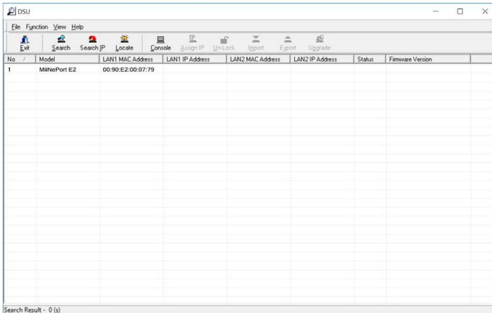
4. To modify the configuration of the highlighted MiiNePort, click the **Console** icon to open the web console. This will take you to the web console, where you can make configuration changes. Refer to **Chapter 7: Web Console Configuration** for information on how to use the web console.
