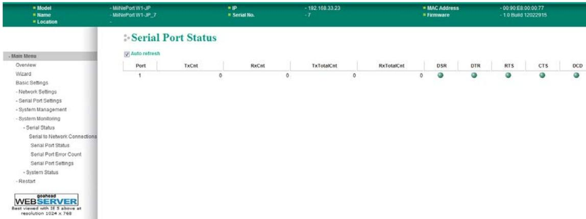
The **Serial Port Status** page is located under **Serial Status** in the **System Monitoring** folder. On this page, you can monitor the serial signal and data transmission status.
