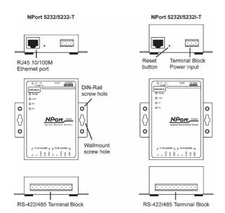
Use the terminal block for both serial interface and power source with a 28 to 12 AWG (torque value minimum 3.5 lb-in/0.5 N.m, maximum 4.4 lb-in/0.5 N.m) cable with the devices.
